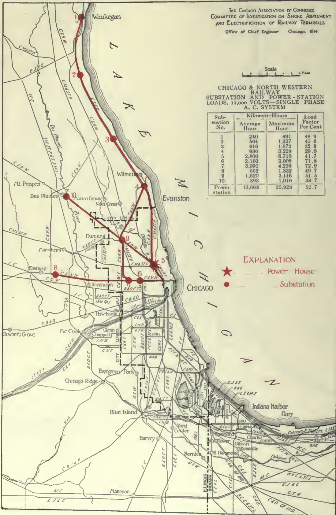
FIG. 625. LOCATIONS OF POWER STATION AND SUBSTATIONS FOR THE CHICAGO & NORTH WESTERN RAILWAY FOR THE 11,000-VOLT A. C. SYSTEM
